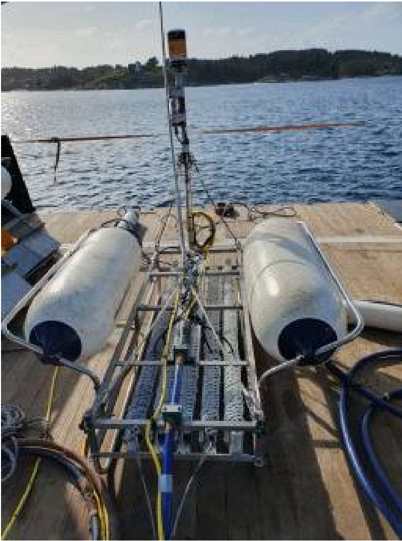
Figure 4. The sparker source used in the current study (photo: Kate McQueen). Two such sources were used together for the sparker treatments.
