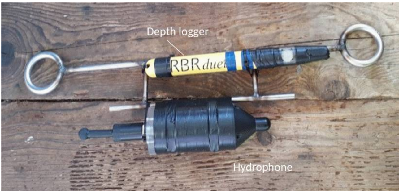
Figure 7. The sound trap hydrophone.
