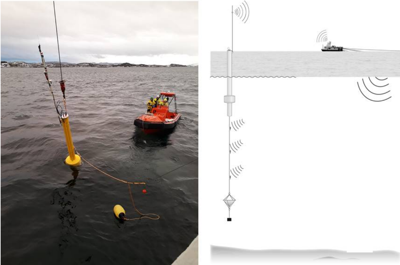
Figure 5. The hydrophone vertical array. Left: The surface part of the array visible above sea level. The array was towed by the HUS workboat into position and moored to the bottom with heavy weights. Right: figure of how it looks when deployed. The figure shows 3 hydrophones at different depths, but in the current setting only two were used and the array was not drifting but fixed at one position.
