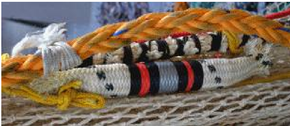
Figure 9.2 – a depth sensor (SXL-0154) in its protective housing and sheath fixed to the top of the FRS.
