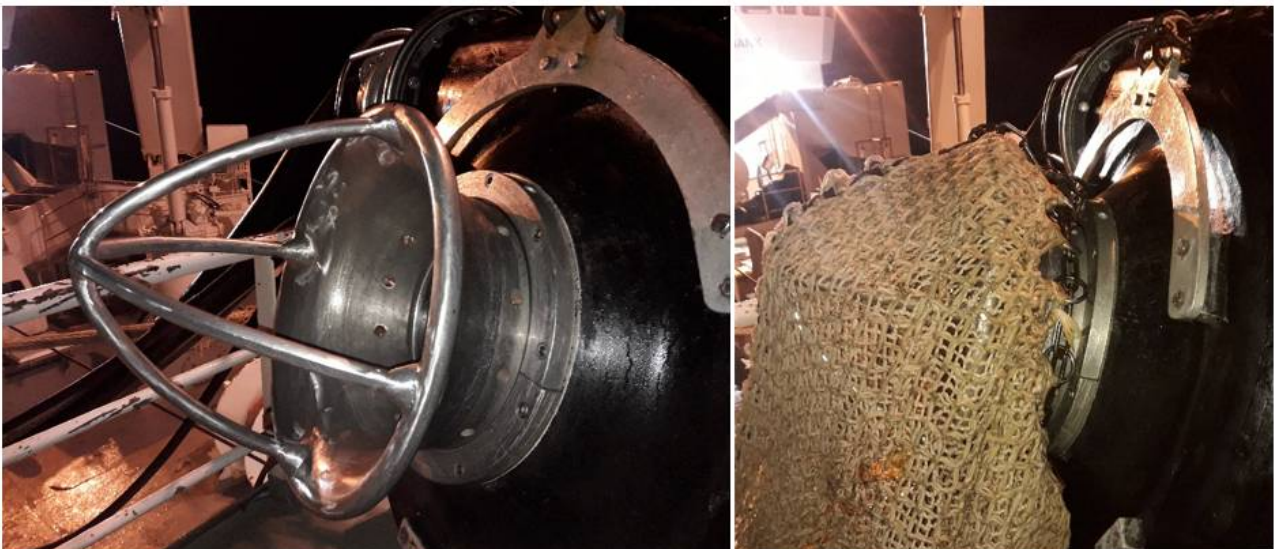
Figure 7.1 - Left: the pump-head funnel; and Right: pump with pump skirt connected [Source: J. Saltskår].
