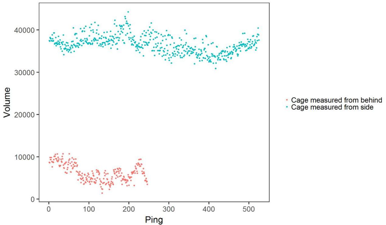
Figure 6. Volume ( $m^3$ ) of tuna in the cage as measured by the sonar and data processed with the LSSS Promus module. Red dots are measurements made from behind the cage and blue dots are from the side.
