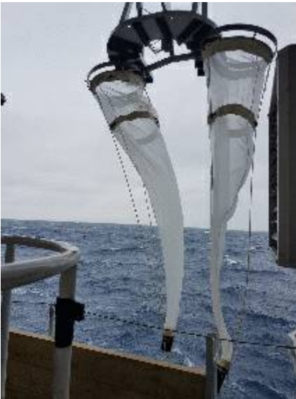
Figure 3.2. The WP2 DUO deployment from the CTD hangar of RV Kronprins Haakon 14 March 2019. Foto: Tone Falkenhaus, IMR.
