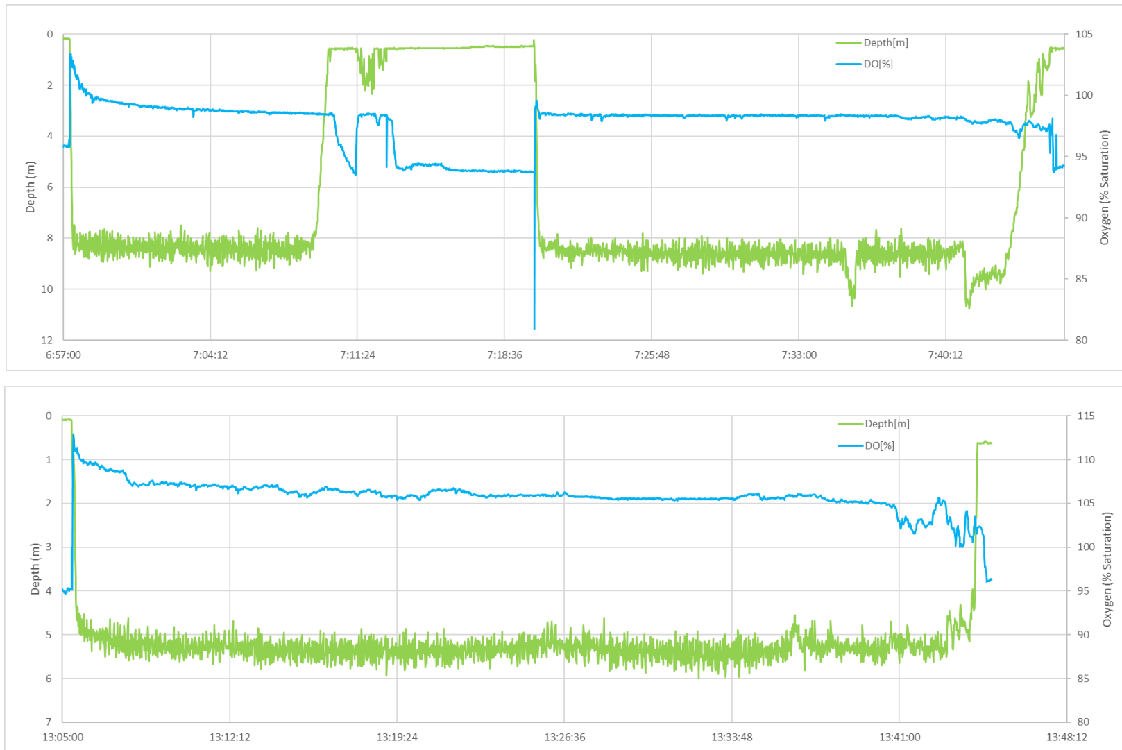
Figure 4.2. Examples of oxygen and depth profiles from the catch monitoring probe (CMP); top cast 01 and bottom cast 09.
