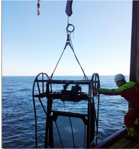
MOCNESS for vertically stratified samples of zooplankton.
