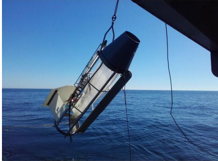
Gulf VII high-speed plankton sampler with PUP net for sampling fish eggs and larvae.
