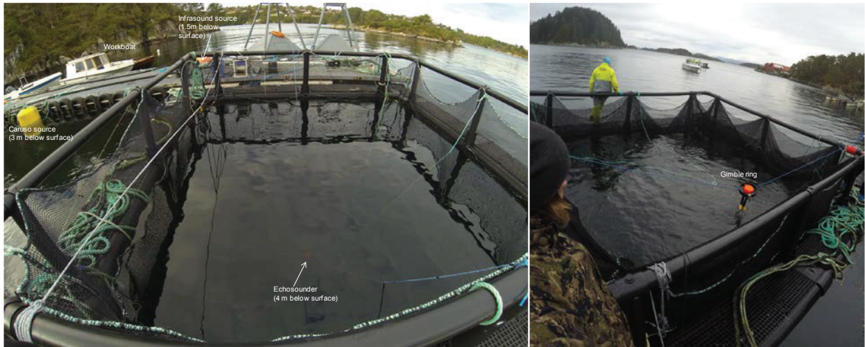
Figure 4. Left: Net pen with the echosounder at depth, visible as an orange ring. Placement of the two sound sources and the workboat were recording or echosounder, ARIS and hydrophone data were done. Right: The echosounder was mounted in a gimble ring, to make it stable under water. Here lifted to the surface. The go-pro camera was also mounted on this ring.
