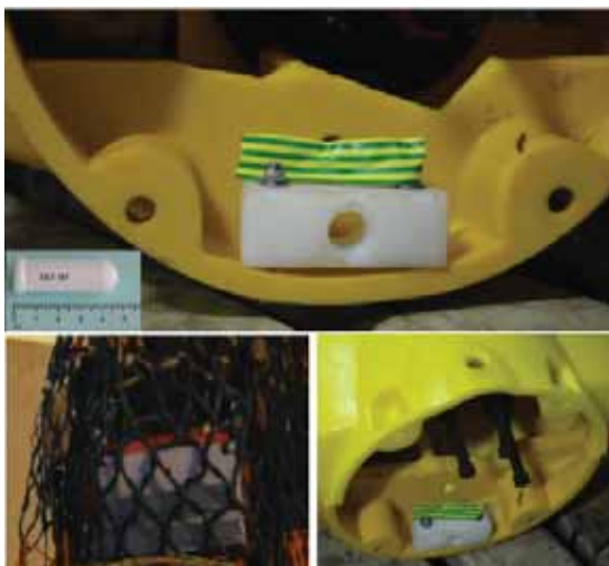
Figure 4. The DST tilt sensors and holders.
