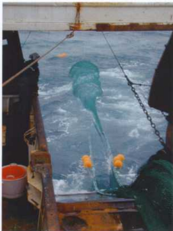
Figure 8. The collection cage floating at the surface as the trawl is set
