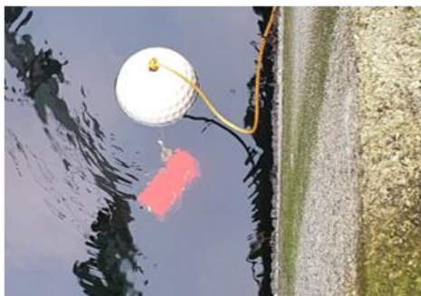
Figure 2: A door sensor (orange rectangle) at 1m depth at the stern of the vessel.
