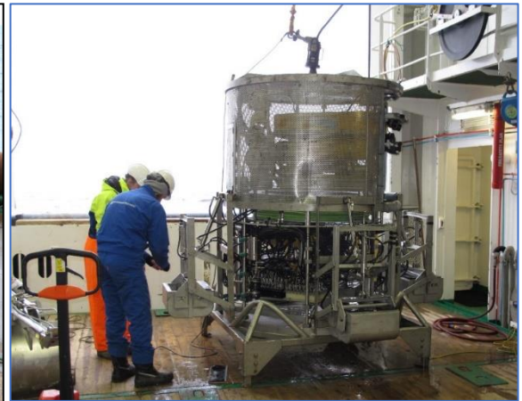
The VAMS rig with its ROV placed within the parking chamber.
