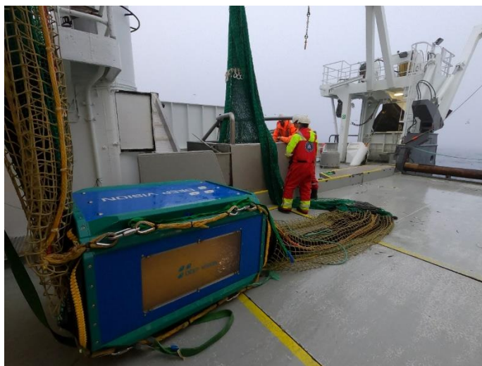
Figure 2.2.5.1 The DeepVision box mounted on an extension in front of the codend.
